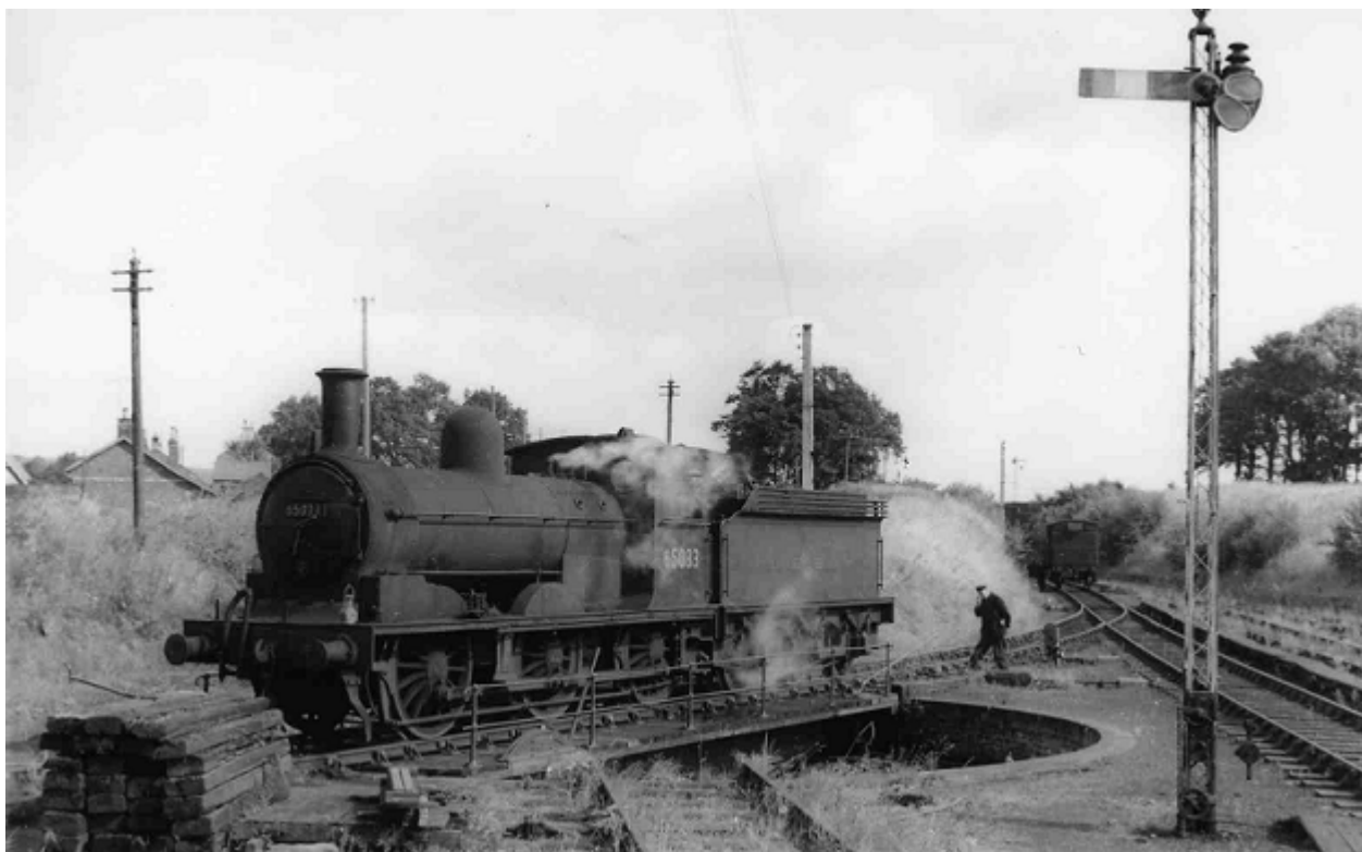
With J21 0-6-0 65033 on the turntable at Reedsmouth, Jimmy Hedley checks that the tender wheels are clear before turning the engine for its return, August 1961.
