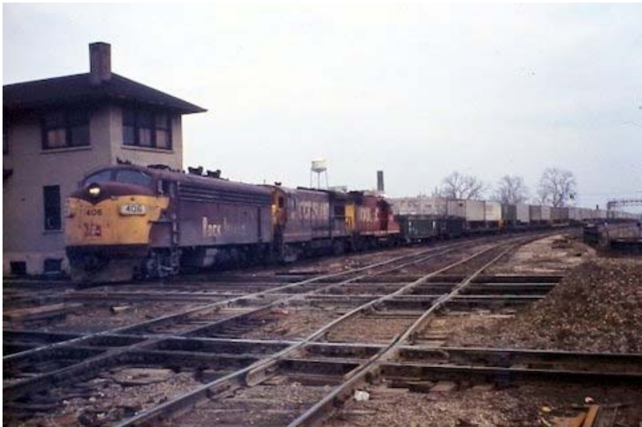
Westbound Rock Island trailer train at Joliet, Illinois, led by EMD FP7 406. Note the state of the Rock Island tracks which still carried the high speed Rock Island and Pretoria Rocket passenger trains; February 1974.
