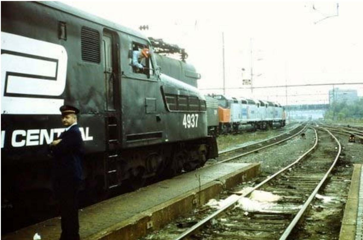
Ex-Pennsylvania Rail Road GG1 electric – fine example of the 1930s Raymond Loewy design – relieves SDP40F and E unit power on the ‘Broadway Limited’ at Harrisburg, Pennsylvania; 15 September 1974.
